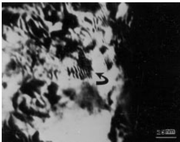
Fig. 8 Moiré patterns indicating the presence of copper clusters in steel C aged at 450 °C, thin foil
